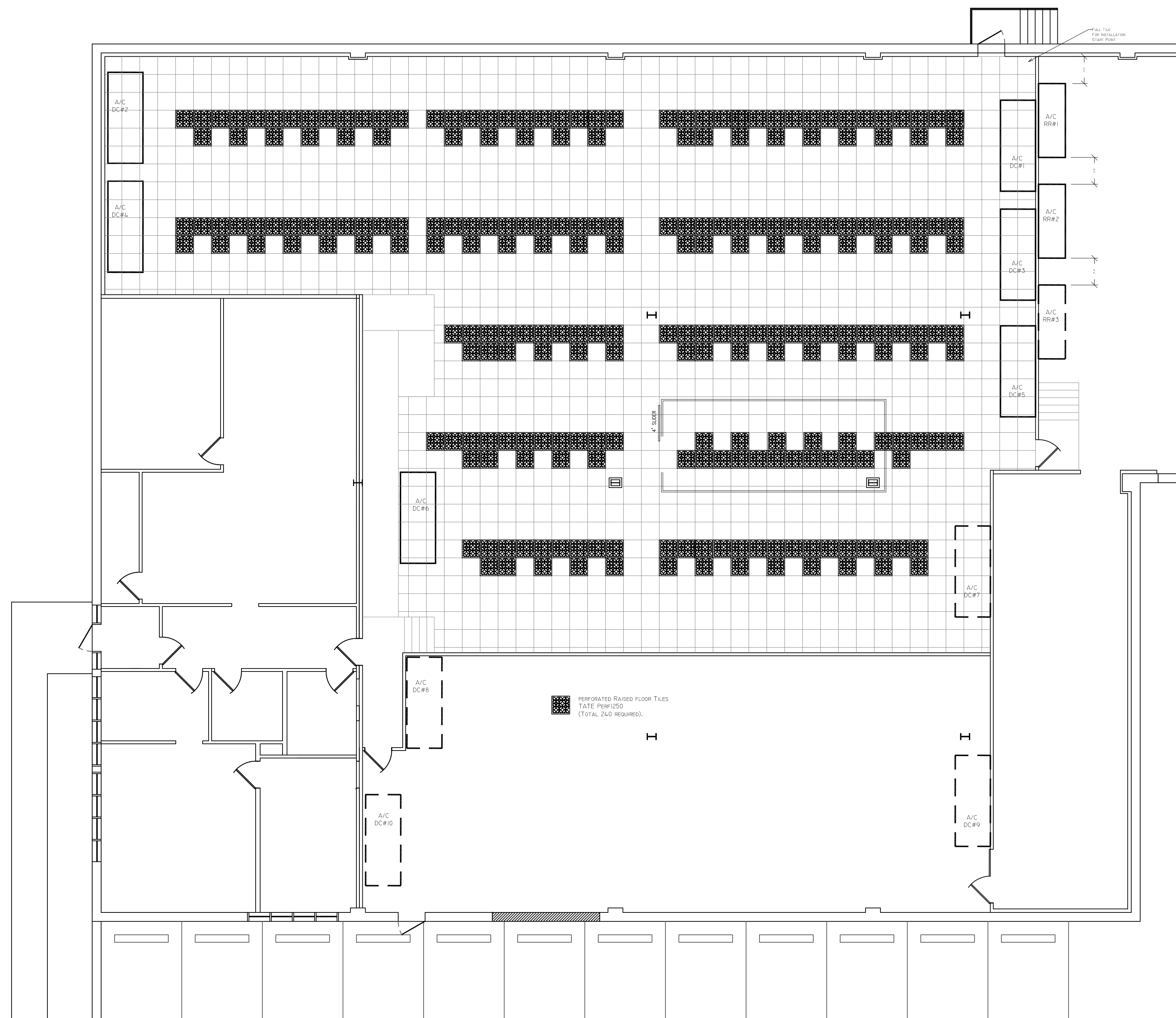
Perforated Floor Tiles Layout Plan
